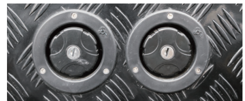
Fig. 3-14 Water Filling Ports of Drinking Water Tank and Purified Water Tank
